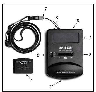
1 – Rechargeable Battery: (Model SA1505) 2.4 volt that will run approximately four hours without recharging. Recharging time is approximately 2.5 hours using Sound Associates SA1905-03 Drop-in Charger or SA1930 Drop-in Multi-charger (each sold separately).
