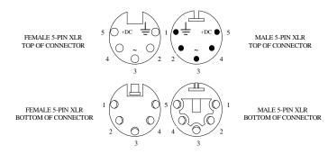
Pin 1: Shield = Ground Pin 2: Ground Pin 3: White / Red = Signal Pin 4: Positive DC Pin 5: Black = Positive DC
