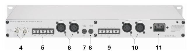
**4 – Modulated Audio Input/Output:** BNC connection allows input to receive modulated audio signal from infrared transmitter and output to link to additional power supplies via RG58u cable (RG59u can be used cable for short runs). Input and output are independent of power source.
