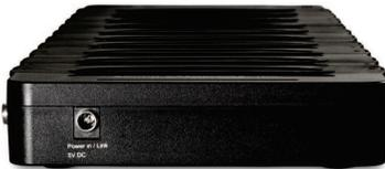
END VIEW: Multiple power connectors to couple two chargers to one power supply
