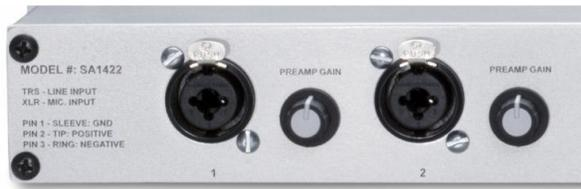
The Neutrik Combo connector accepts a balanced XLR line connector or a ¼" phone plug. The XLR connector is wired with **pin 1** as **ground**, **pin 2** as **positive (+)**, and **pin 3** as **negative (-)**. The ¼" phone plug is wired with the **sleeve** as **ground**, the **ring** as **negative (-)**, and the **tip** as **positive (+)**. Use the pre-amp gain control to best match the audio level of the source.
