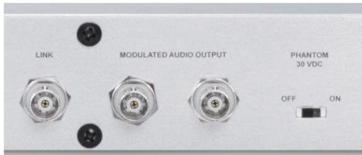
The link connection on the back of the SA1422 allows 2 transmitters to be linked together to utilize up to four channels of transmission. The unit which utilizes 2 channels should be the first in line. The second can utilize 1 or 2 channels. The emitter power supply or emitter panels must be connected to the second or last transmitter in the string. This will allow for proper output voltage to the emitters. See example diagram on the following page:
