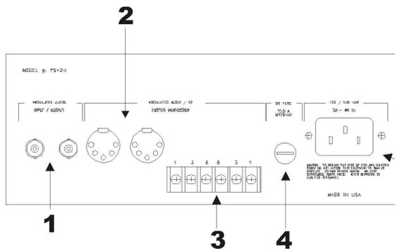
**1 – Modulated Audio Input/Output:** BNC connection allows input to receive modulated audio signal from infrared transmitter and output to link to additional power supplies via RG58u cable (RG59u cable for short runs).
