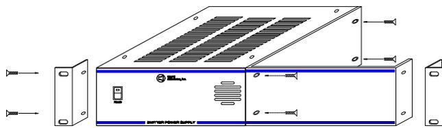
To mount a single power supply in a standard 19" rack, use a RK1 single rack mount kit. Fix the blank half space bracket to the side of the power supply with the four enclosed flat head 8/32 screws (see figure). Attach the rack ears to the power supply and to the blank panel with the four enclosed flat head 8/32 screws. All screw lengths should not exceed 1/2 inch.
