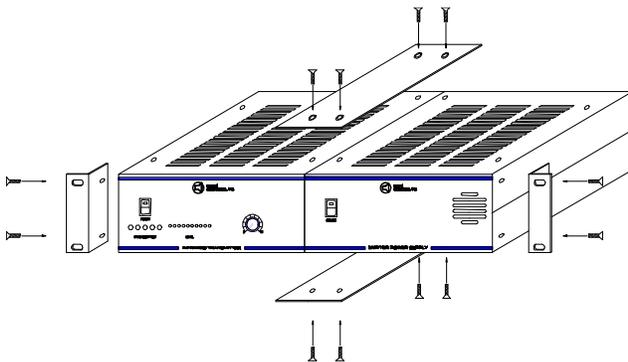
To mount two emitter power supplies or a transmitter and emitter power supply side by side in a standard 19" rack, use a RK2 double rack mount kit. Place the power supplies or transmitter and power supply side by side on a flat surface. Fix the top support plate to the units with four flat head 8/32 screws (see figure on previous page). Once the support plate is tightened, flip the units and attach the bottom support plate with four flat head 8/32 screws, then attach
