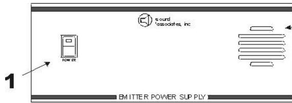
**1 – Power Switch:** Applies line power. Rocker switch with LED to indicate on/off modes. The LED on switch also indicates DC voltage is present. If LED on switch does not light, check if AC power and DC power are working properly.
