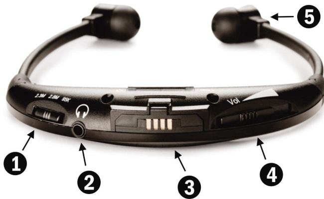
**1 – Channel Selector:** (Model SA1523H only) The recessed selector button toggles to one of three positions: 2.3 MHz (left), 2.8 MHz (center), and 95 kHz (right).
